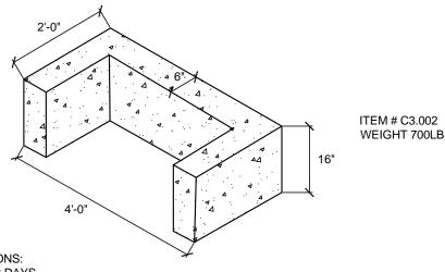
SPECIFICATIONS: 5000 psi AT 28 DAYS REINFORCING- 2X2X12 GAUGE W.W.M AIR ENTRAINING 5-7%
