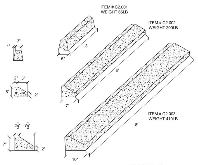
SPECIFICATIONS: 5000 psi AT 28 DAYS AIR ENTRAINING 5-7% 10mm REBAR REINFORCING
