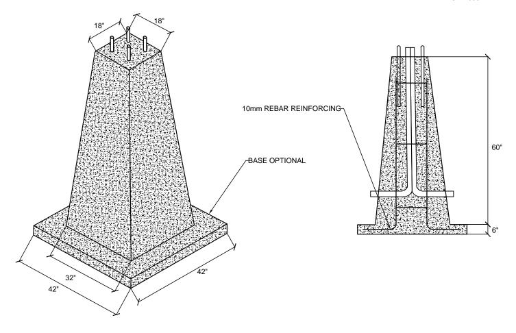
SPECIFICATIONS: 5000 psi AT 28 DAYS AIR ENTRAINING 5-7% 10mm REBAR REINFORCING CONDUIT SIZE AND LOCATION AS PER CUSTOMER SPECIFICATIONS
