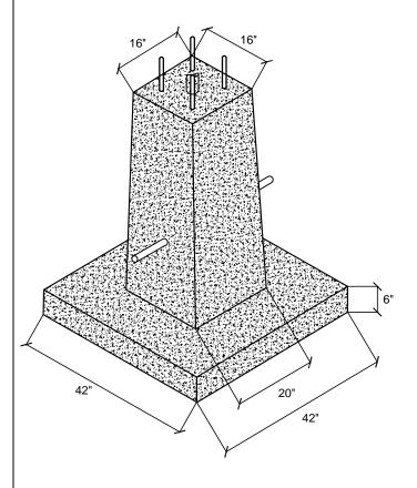
10mm REBAR REINFORCING
