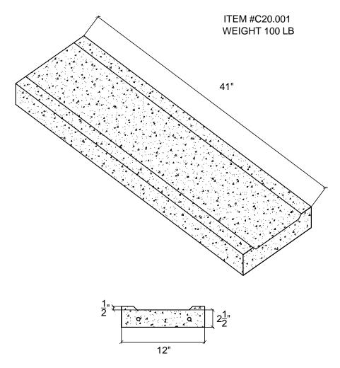
SPECIFICATIONS: 5000 psi AT 28 DAYS REINFORCING AS SHOWN BELOW AIR ENTRAINING 5-7%
