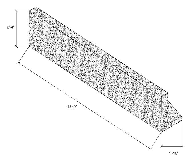
SPECIFICATIONS: 5000 psi AT 28 DAYS AIR ENTRAINING 5-7% 10mm REBAR REINFORCING
