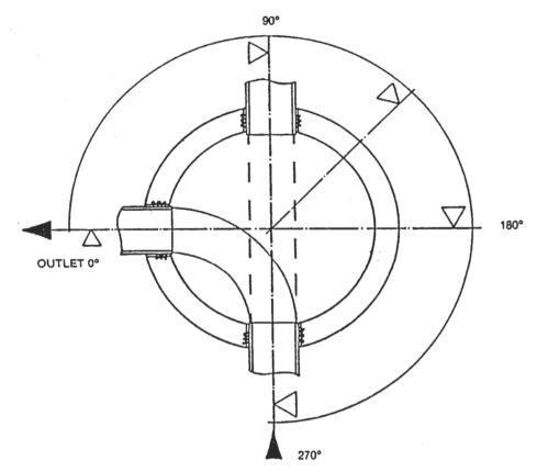
NOTE: Holes available in 5° increments from 90° to 270°. The outlet hole is denoted 0° and the inlet is measured in a clockwise direction from the outlet (shown above).
